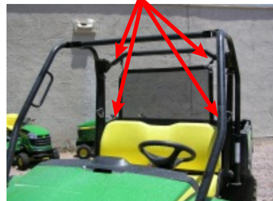
Shock Cords installed in eyelet and then around wide ROPS and clipped back onto the Shock Cord
