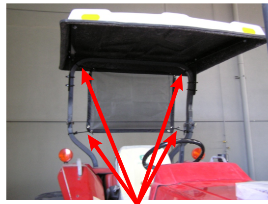
Shock Cords installed in eyelet and then around wide ROPS and clipped back onto the Shock Cord
